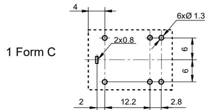
Remark: 1) In case of no tolerance shown in outline dimension: outline dimension  $\leq 1\text{mm}$ , tolerance should be  $\pm 0.2\text{mm}$ ; outline dimension  $> 1\text{mm}$  and  $\leq 5\text{mm}$ , tolerance should be  $\pm 0.3\text{mm}$ ; outline dimension  $> 5\text{mm}$ , tolerance should be  $\pm 0.4\text{mm}$ .
